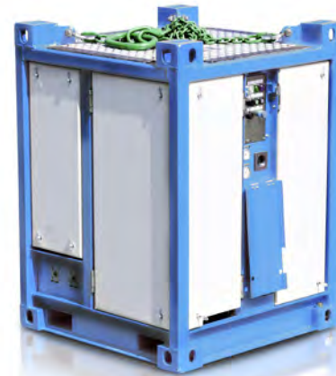
High pressure, hot water wash down system for Zone 1 hazardous area. 300 bar and 16 l/min. DNV 2.7-1 approved.
